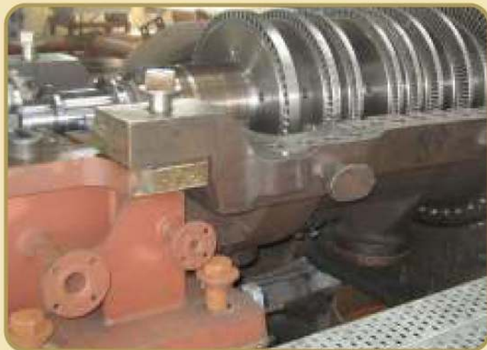
Steam Turbine under assembly
