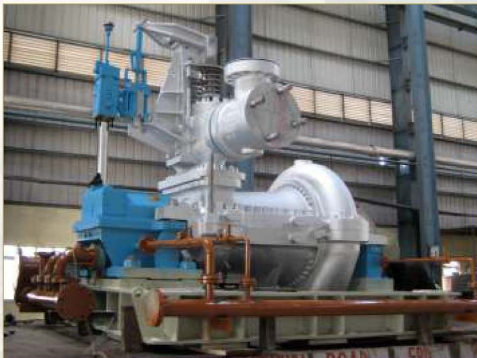
8MW Steam Turbine
